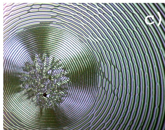
FIG. 7. (Color online) (a) Temporal evolution of the buckling instability of the droplet chains, T=122 °C for (a) 31 min, (b) 39 min, (c) 85 min after the beginning of illumination, width of the images is 859.6 \mu\text{m} . The inner rings are first filled up by droplets and start buckling with a distinct wavelength. Later, the outer rings are filled up.
